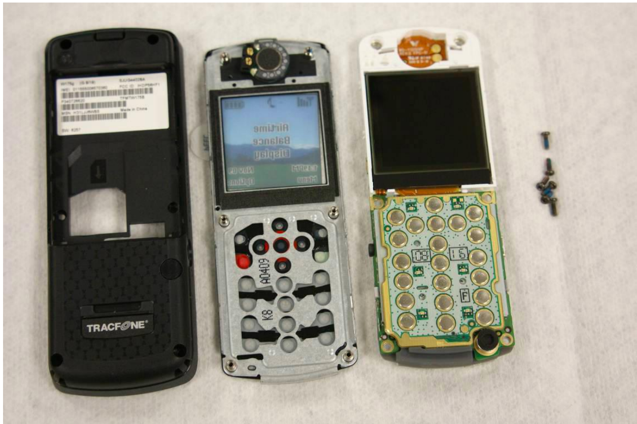
Figure 4. Three major components of the W175g handset: back-cover with identification label, front cover with speaker and touchpad assembly, and main circuit board with attached switches for keyboard and Liquid Crystal Display unit.
