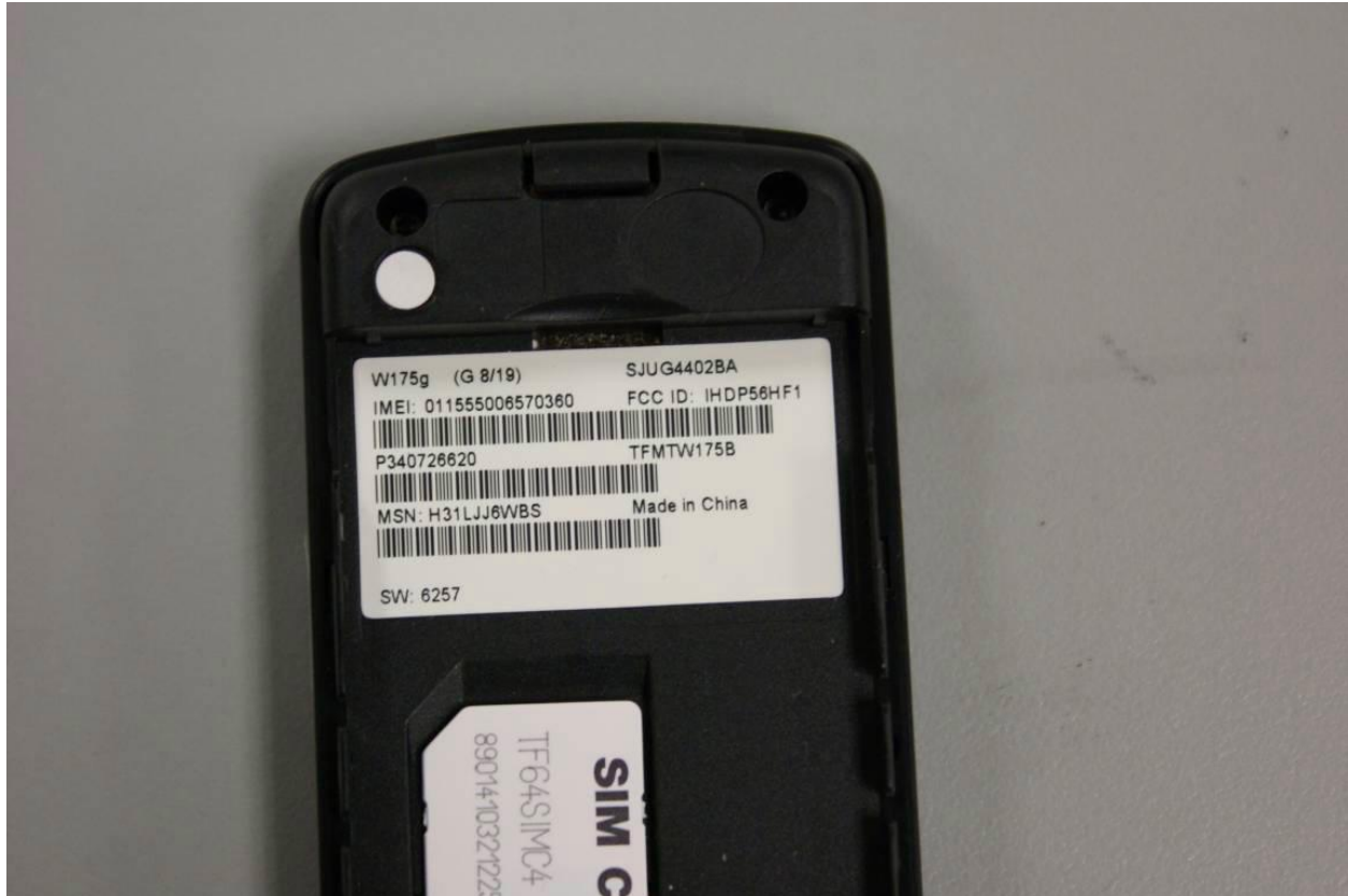
Figure 3. Photograph of identification label attached to the disassembled cellular handset.
