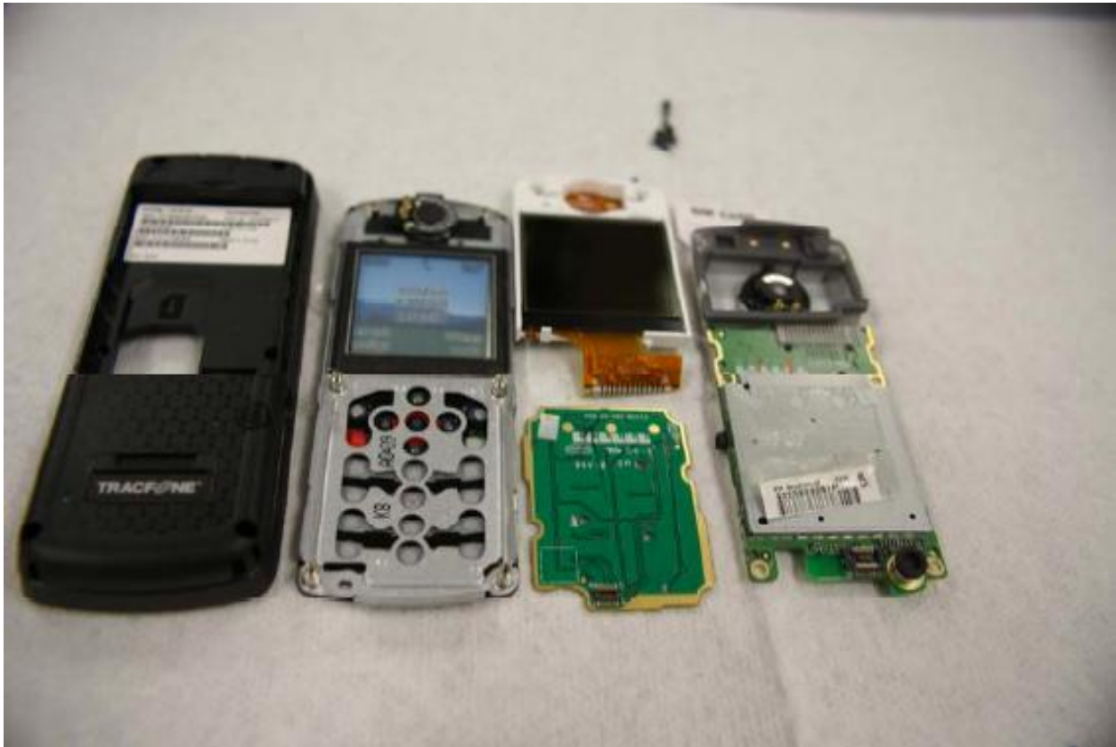
Figure 5. Major components of the W175g handset: cover, speaker/keyboard module, PCB with heat sink, and LCD display.
